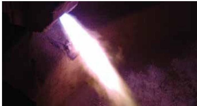
Stable and hot flame close to the injector tip.
