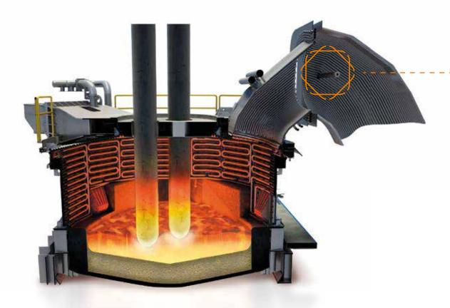
The innovative **LINDARC™ EVO** off-gas analysis technology, installed on the fix duct uses the innovative technique of "Multiplexed Tunable Diode Laser Absorption Spectroscopy" (WM-TDLAS) which combines lasers and fiber-optics to obtain exact data of various gas species in the EAF off-gas system in real time.
