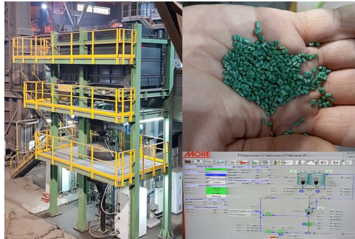
Fig 14 Integrated plant for polymer and coke mixing and injecting into EAF, Tenaris Silcotub 2021
