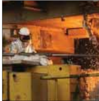
Fig 3 Operator lancing the taphole
