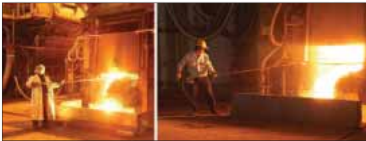
🕒 Fig 2 Operators taking a sample or a probe
